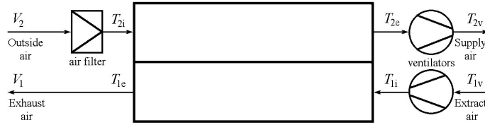
Fig. 5. Schematic representation of a compact ventilation system unit for single or multiple dwelling airing
